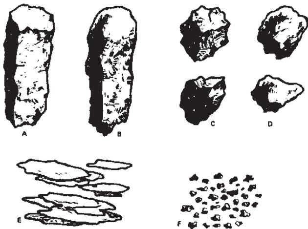
Figure 4. Drawings illustrate some of the types of soil structure: A—prismatic; B—columnar; C—angular blocky; D—subangular blocky; E—platy; and F—granular.
