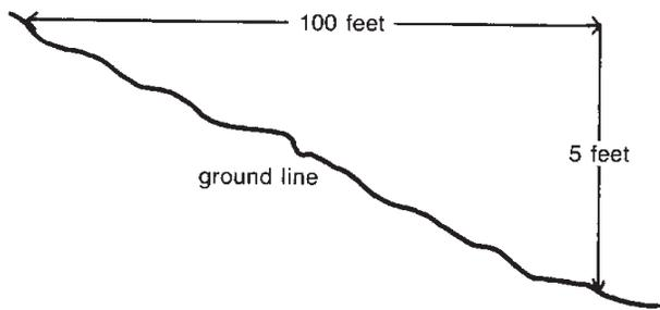
Figure 3. Diagram showing a 5 percent slope.
